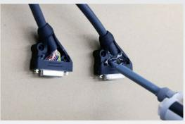
During the final assembly, the pre-assembled plug-cable combination is inserted into the lower part of the housing, encapsulated with a 2K mass and then sealed.
